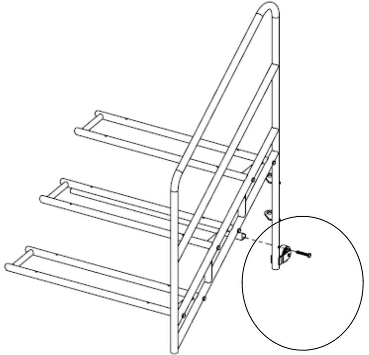
Repeat the same process on the left side of the unit by aligning the ends of the metal step frames and the cross brace with the holes on the second guardrail. Use 7— M10 bolts and washers to attach all three metal step frames and cross brace.
