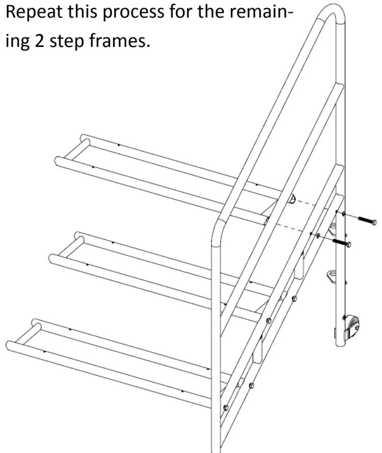
Locate the long cross brace and begin to align the end of the brace to the hole on the guardrail as shown in the illustration. Once the end of the cross brace is aligned, place a washer on an M10 bolt and attach the brace to the guardrail by threading the bolt through the guardrail and into the end of the brace.
