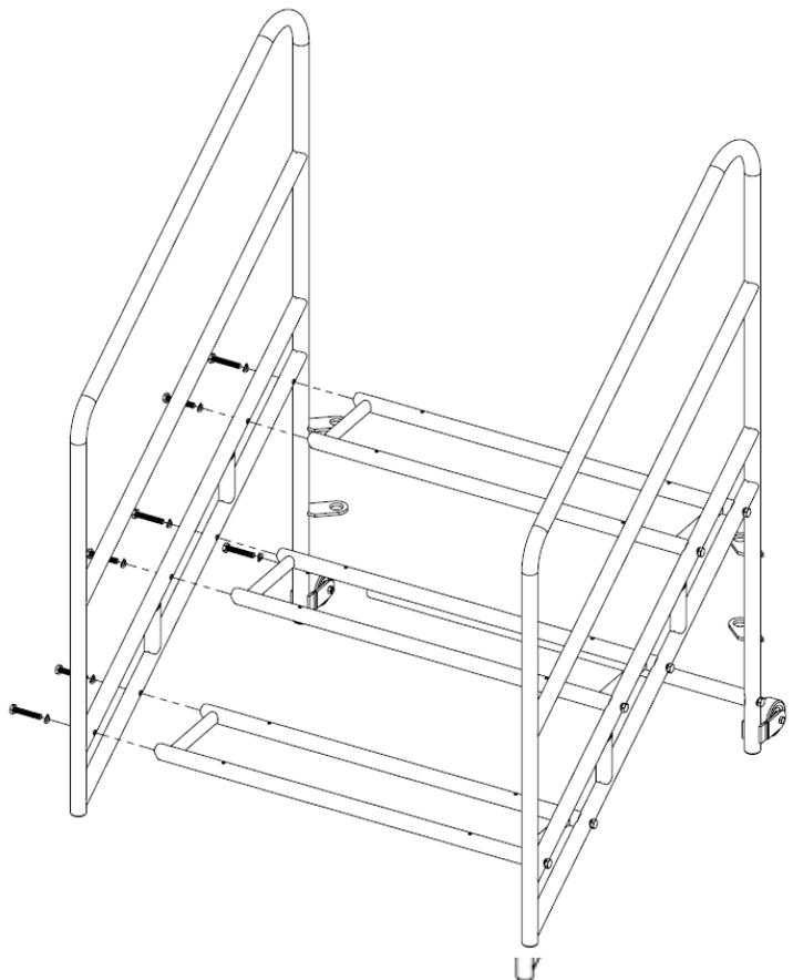
Use a proper wrench to tighten all the bolts to ensure that the unit is stable.
