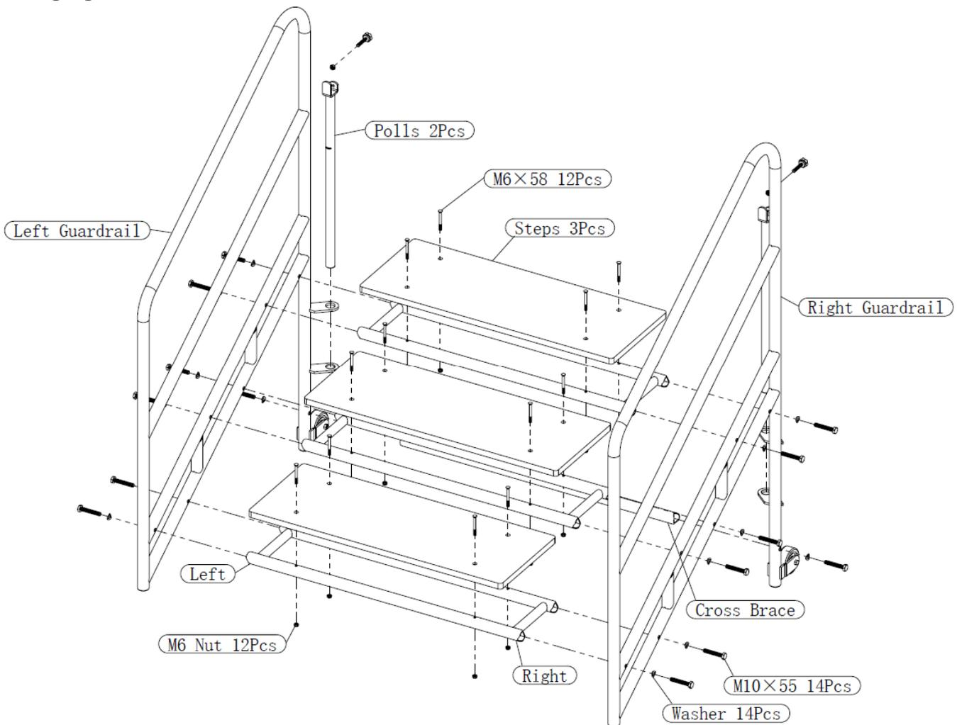
Note that one guardrail is labeled “R” for right and one guardrail is labeled “L” for Left. In addition there are labels at each end of the metal step frame identifying right & left sides.
